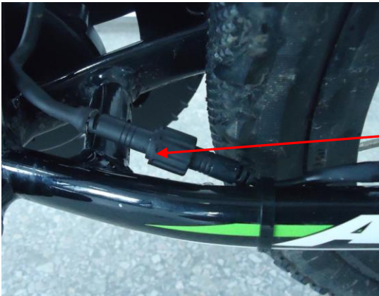
Water proof connector for speed detecting sensor
