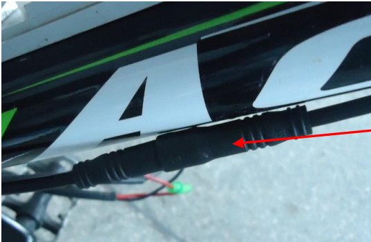
Water proof connector for display
